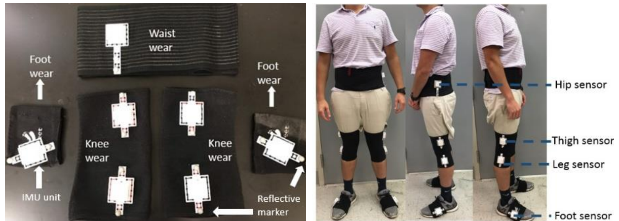
Figure 9-1: (a) shows the overview of the tracking system with reflective markers, and (b) suggested mounting locations on the hip, knees, and ankles of end-users. The IMU modules were placed on the outer surface of the hip, knees, and ankles.
